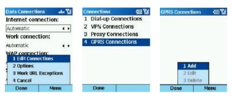
Fill out the information, Fill "VirginMMS" under Description Connects to "Work", Access point is "VirginMMS" Leave all other fields blank.
